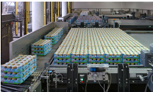
Multiline palletising system for cases of frozen vegetables
